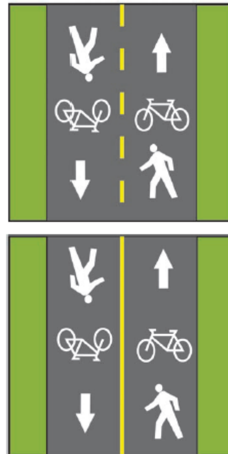
Figure 4.98 – Typical Pavement Markings for Two-Way In-Boulevard Shared Use Paths (Broken versus solid yellow centre line)
